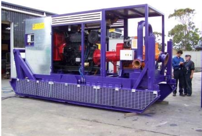
PCE736 Current photo - H/D mine dewatering setup
